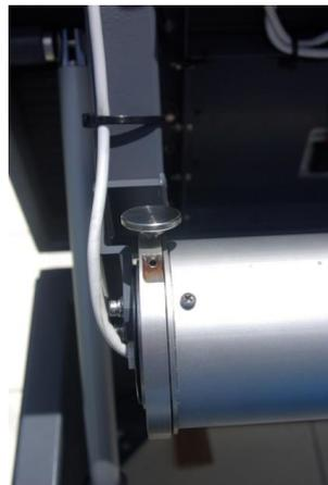
24. Disengage drive motor (to free wheel) – pull up (slight tube rotation may be needed to take weight off pin)
