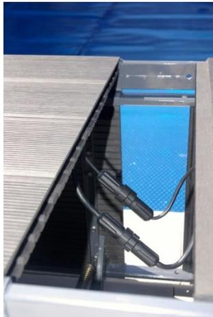
8. Join cables then slide fully together so bolt holes line up (you may need to slightly 'jiggle' up and down or side to side to walk the connectors together, not too much or they will jam)
