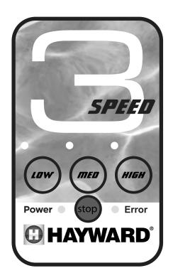
Press and hold , , or for aproximatly three (3) seconds or untill the LED of the selected speed begins to flash. Once flashing the selected speed has entered into the Adjustable Set Point Mode. To reset the speeds to the factory default settings hold down all three (3) buttons untill all three LED's are solidly lit.
