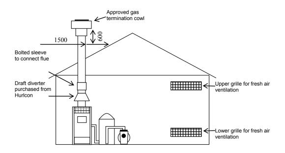
An indoor draught diverter must be purchased from Hurlcon and fitted to unit in accordance with Hurlcon's Instructions and Installation Codes before the heater can be enclosed.
