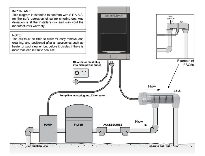
Two self-tapping screws and wall plugs have been provided for fast and simple installation. Simply cut out Template at bottom of page 19 for location of drill entry points. Use a 7mm masonry drill bit when fitting Power Supply to a brick or concrete wall. When mounting to a post drill pilot holes and fit screws provided. Once screws are in position simply hang chlorinator via bracket on back of Unit.
