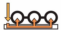
The water channels are in direct contact with the roofing material. This ensures rapid and efficient transfer of heat from the roof to the water.
