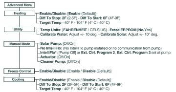
Note: (\*) Only displays if IntelliFlo pump if connected and communicating with SolarTouch controller. Note: (\*\*) **Program 2** is assigned for solar heating/cooling.
