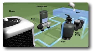
The Electrochlor is plumbed directly in-line with the pool equipment, typically after the heater
