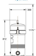
\* Minimum Clearance Height to Remove Cartridge (mm)
